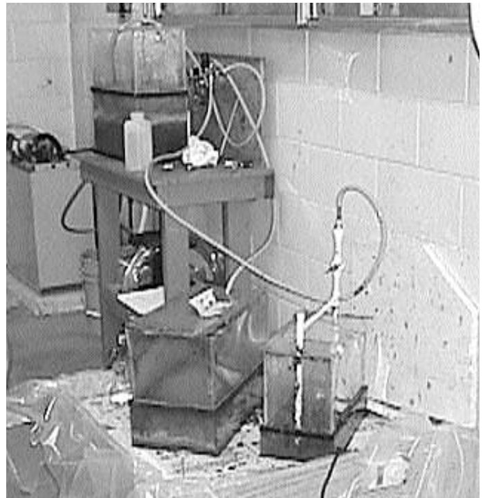
Figure 1—Bench-Scale Aerobic Digestion Test Apparatus
